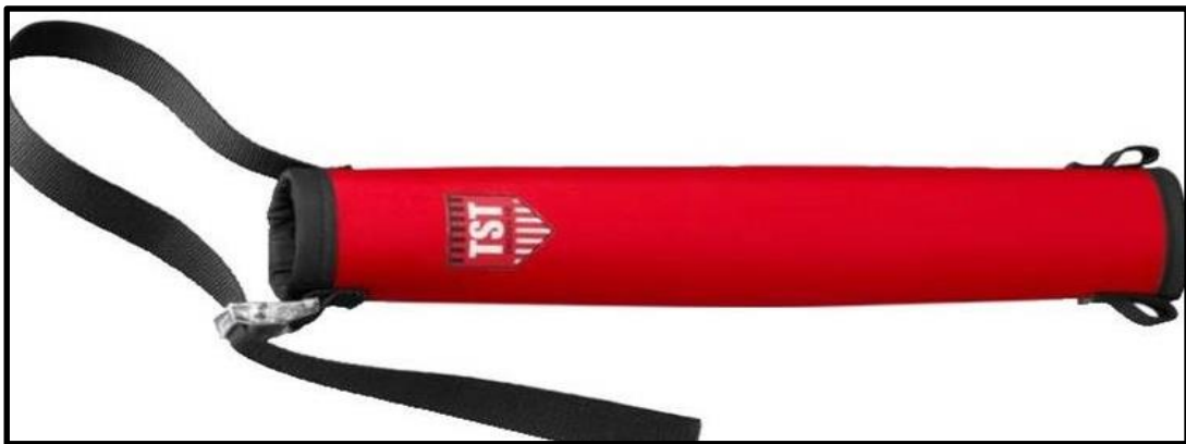
Figure 2 The shroud It is not tested to contain pin hole leaks, designed for hose burst containment at 3000 bar / 43500 psi. Foot pedal shroud. It is NOT intended for use on any hand held equipment.
