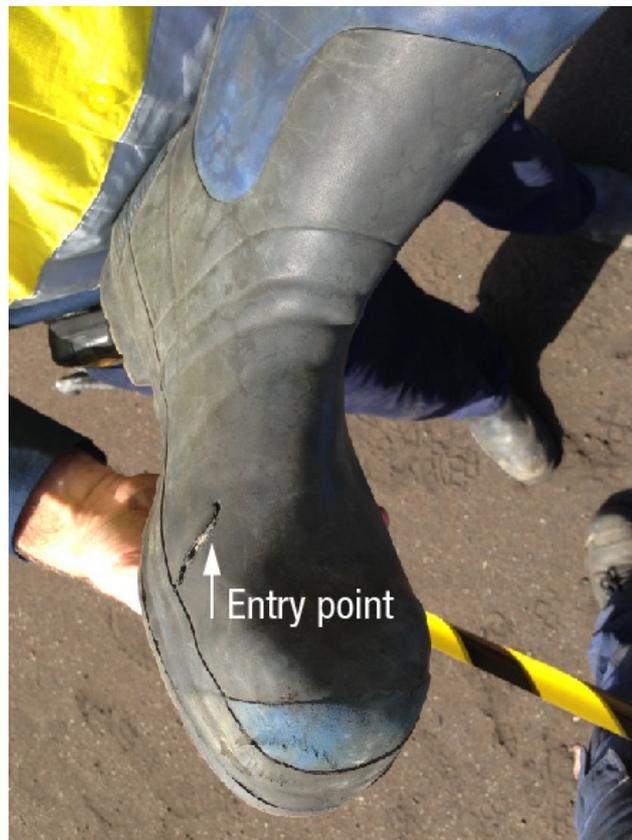
Entry point where high-pressure water jet penetrated boot lining
