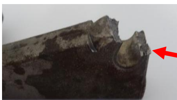
Foot pedal section that snapped during operations.
