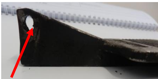
Elongation of pivot hole shown on foot pedal.
