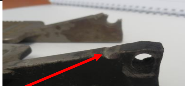
Deep scoring on the top of the foot pedal.
