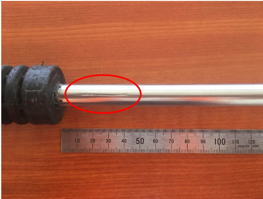
Figure 1: 30mm Split in the Lance Tube.
